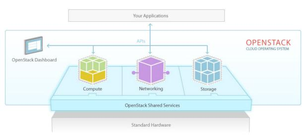
**FIGURE 1. A G**eneral Overview of OpenStack (Image from the OpenStack Project Website)
